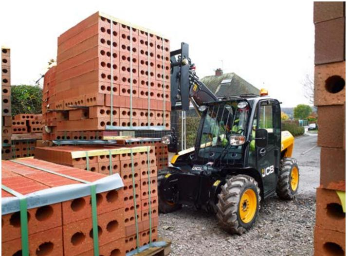
**Our Adaptive Load Control** system automatically prevents machines from tipping forward during heavy load handling.
