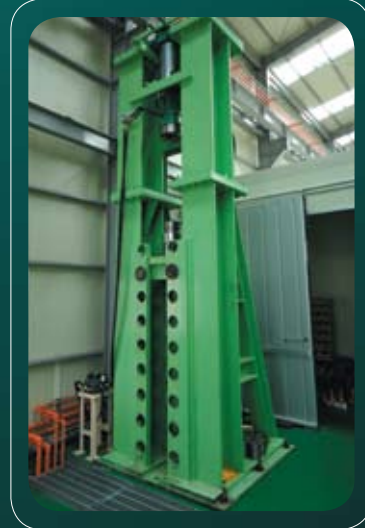
Static calibration test stand for correct measurement.
