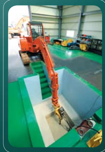
Test unit installed on impact base connected with strain gauge in tool bit and flow and pressure gauge on main hoses.
