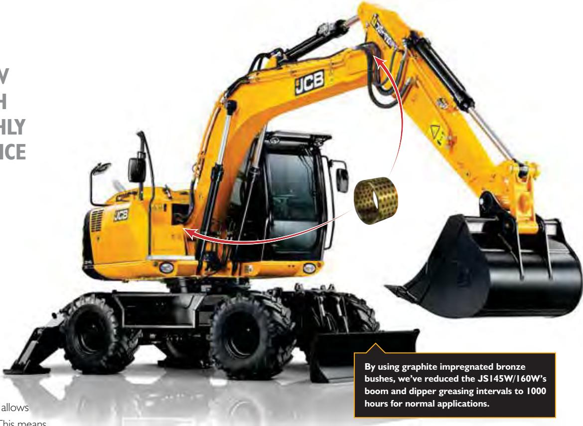
By using graphite impregnated bronze bushes, we've reduced the JS145W/I60W's boom and dipper greasing intervals to 1000 hours for normal applications.
