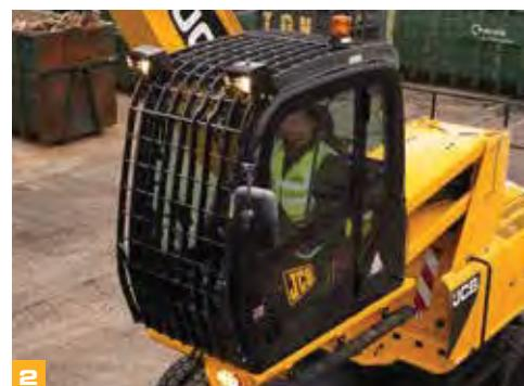
**2** The hydraulic raised cab option enables the raising of the operating station up to 2.3m above the standard machine. This enables the operator to see into higher sided containers that are being loaded, minimising damage, maximising productivity and improving site safety.
