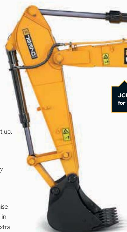
JCB JS330/370 grease points are centralised for safe and easy access to high level pivots.
