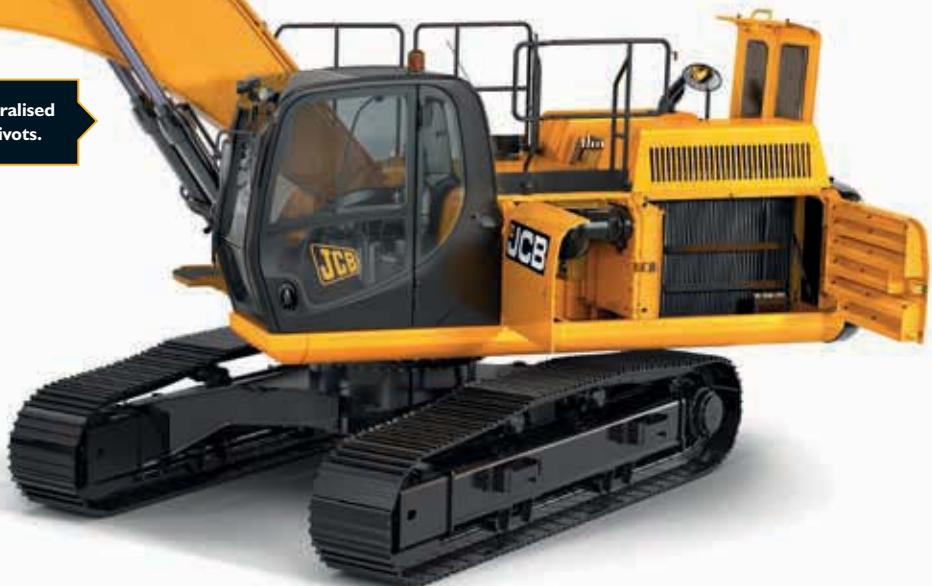
The JCB JS330/370 bonnet opens and closes easily with gas-assisted cylinders, and the service bays are large and wide for good access.
