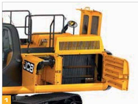
1 JCB JS330/370 bonnet opens front-to-rear for easy and safe engine service access. To make operator access safer, we've installed a tread plate over the engine of the new JS330 and 370. A fuel shut off tap provides a quick, safe way to change fuel filters and reduce the risk of spillage and contamination.
