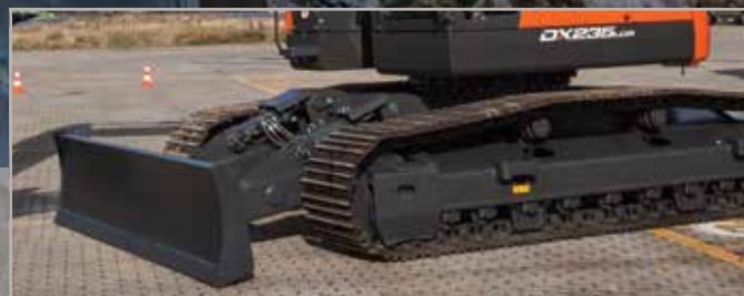
Highly durable dozer blade & undercarriage
