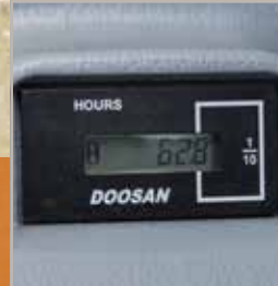
Hour meter (from ground level)
