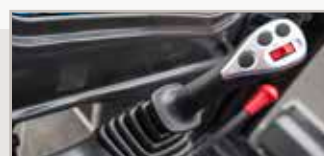
Proportional joystick with auxiliary thumb control
