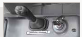
Dozer float function and travel mode switch
