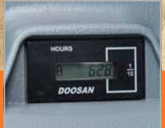
Hour meter (from ground level)
