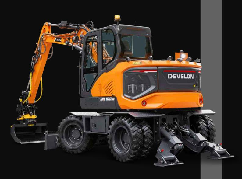
Maximum power 100 hp Operating weight  $10.7^{-11.1}$  t Bucket capacity  $0.28 \text{ m}^3$
